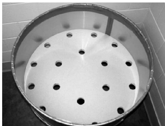
Fig. 3. Odor arena apparatus showing 18 hole positions designed to hold comparison stimulus cups.
